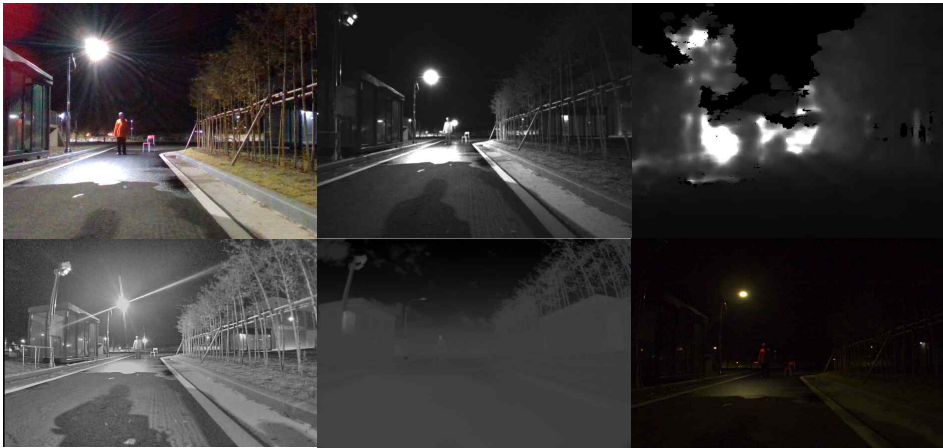
Fig. 11. Multi modal dataset : (Top-Left) RGB(D435) (Top-middle) IR (Top-Right) Depth (Bottom-Left) Night Vision (Bottom-middle) Thermal (Bottom-Right) RGB(Global Shutter)
