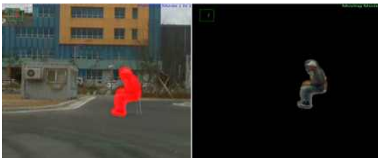
Fig. 7. Result of Pixel Labeling Red Color on the left image is pixel labeling.
