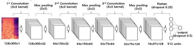
Figure 5. CNN model configuration for cough detection
