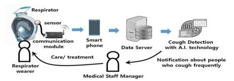
Figure 1. The overall structure of the cough detection system
