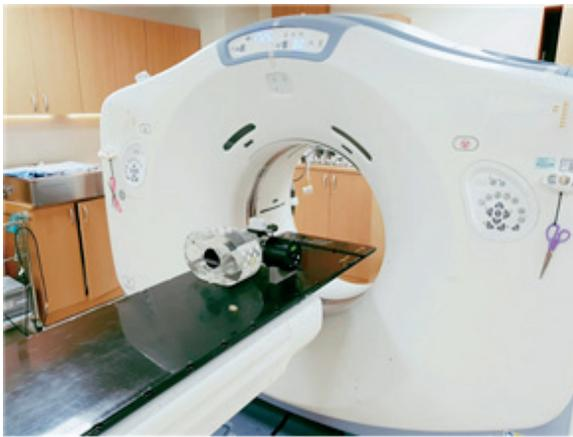
A. CT Simulator for Phantom Study Lightspeed RT16 CT simulator(General Electric Co, USA)
