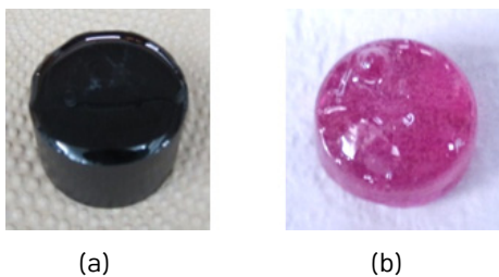
Fig. 1. (a) Rare earths oxide glass waste form, (b) Rare earths phosphate glass waste form.
