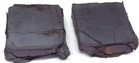
Fig. 1. Collapsed La_{0.33}Sr_{0.67}MnO_3 after the immersion in LiCl-Li_2O molten salt for 7 days, showing the surface delamination.
