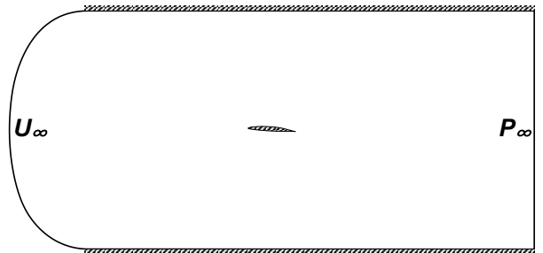
Fig. 2 Computational domain and boundary condition
