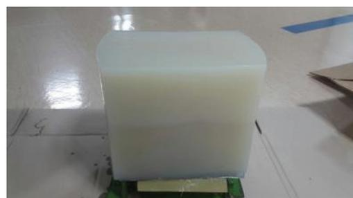
Fig. 2. Agar phantom for analyzing the temperature rise specificity of Hyperthermia device.
