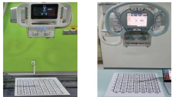
(a) Actual focal angle of anode 12° (b) Actual focal angle of anode 16°
