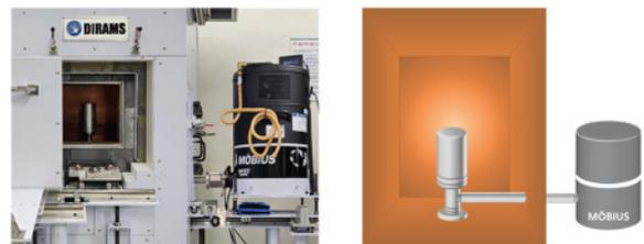
Fig. 1. HPGe (High Purity Germanium) detector.
