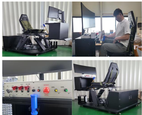
Fig. 11. Finally implemented motion chair
