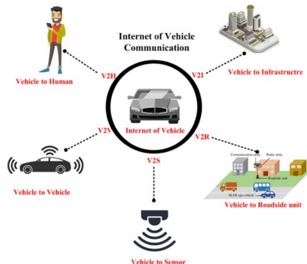
Fig. 1. Five types of network communication in IoV [5]
