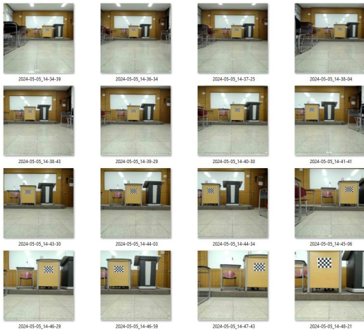
Fig. 4 Test cases for camera position estimation with normal brightness
