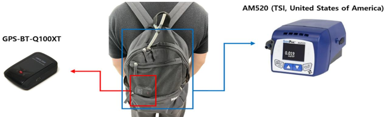
Fig. 1. Measuring instruments used in the active-simulations
