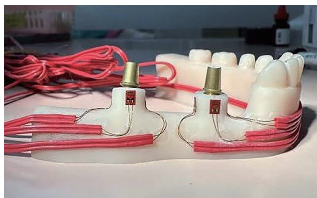
Fig. 4. Location of strain gauges on the model.
