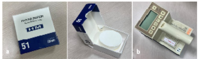
Fig. 2. (a) Smear paper (Hyundai micro, Korea), (b) Surface Contamination Monitor (EBERLINE, Erlangen)
