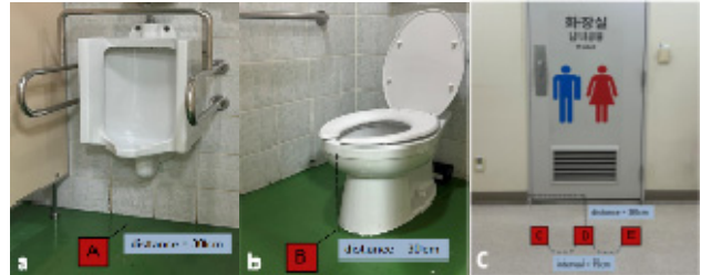
Fig. 1. (a) Measurement area at restroom of \gamma -camera room (Urinal), (b) Measurement area at restroom of PET room-Iodine treatment room(Toilet), (c) Measurement area at entrance of restroom
