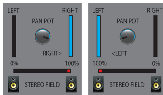
Fig. 1. (Color available online) Example image of stereophonic panning function inside of a Digital Audio Workstation (DAW) program. The left image shows the panning hard left and the right image shows the opposite with corresponding gain strength (light blue color).
