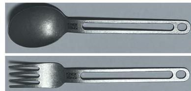
Fig. 15. Products that are labeled as STS 316 grade, but are suspected to be STS 304 grade spoon(up) and fork(down)
