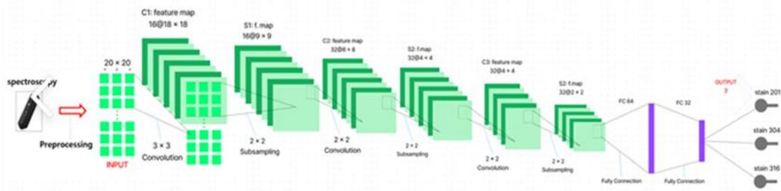
Fig. 9. CNN Model to classify STS grades
