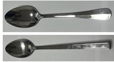
Fig. 13. STS 304 grade product used for testing
