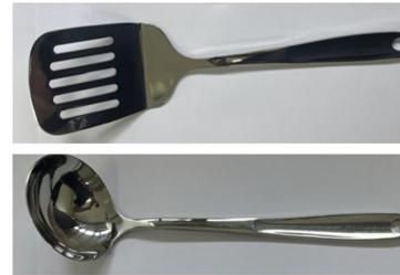
Fig. 14. STS 316 grade product used for testing
