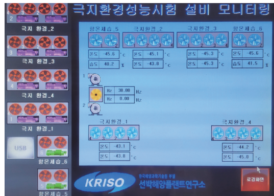
Fig. 8 Temperature deviation at -45 degree setting
