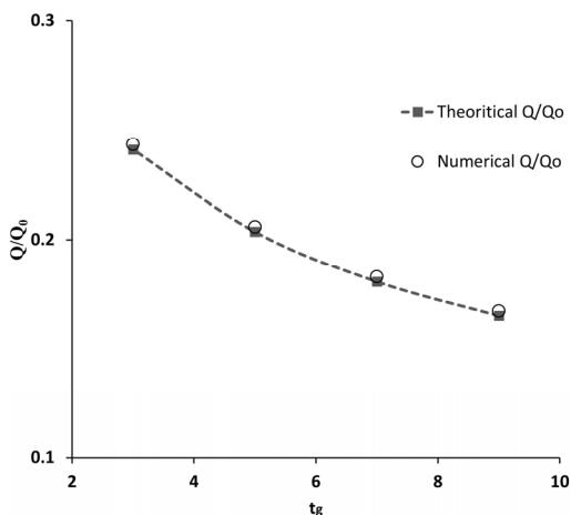
Fig. 14. Effect of grout thickness ( $k_g/k_s = 0.1$ ) on water inflow
