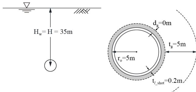
Fig. 6. Representative section of parametric analysis
