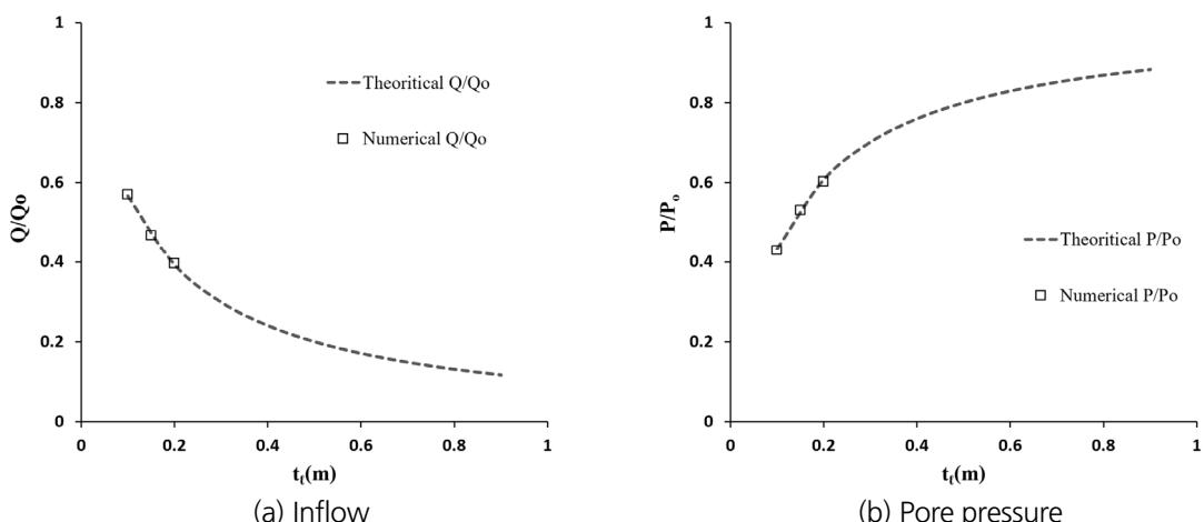
Fig. 16. Effect of excavation support thickness ( $k_l/k_s = 0.01$ ) on water inflow
