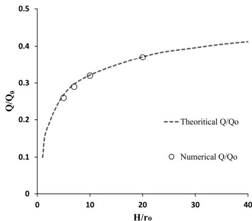
Fig. 13. Effect of tunnel depth ( $k_g/k_s = 0.1$ ,  $t_g = 5$  m) on water inflow
