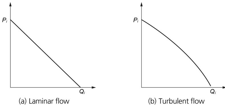
Fig. 1. Tunnel hydraulic boundary conditions (Joo and Shin, 2014)
