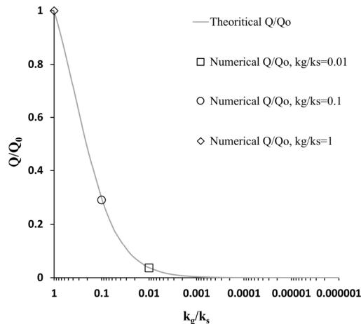
Fig. 15. Effect of  $k_g/k_s$  ( $t_g = 5$  m) on water inflow
