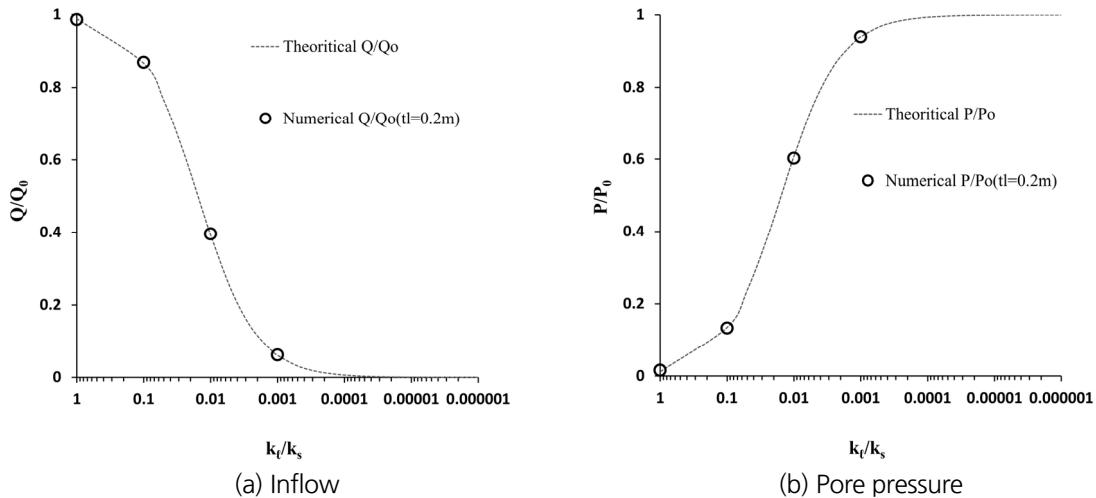
Fig. 17. Effect of  $k_l/k_s$  ( $t_l = 0.2$  m) on water inflow
