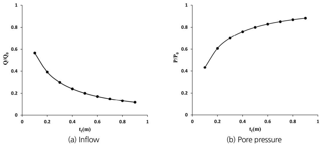
Fig. 10. Effect of support thickness ( $k_l/k_s = 0.01$ ) on water inflow
