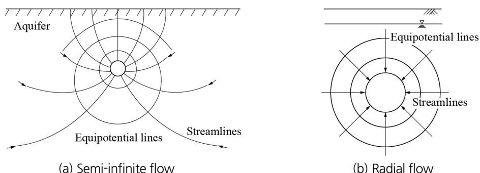
Fig. 2. Flow conditions for tunnelling
