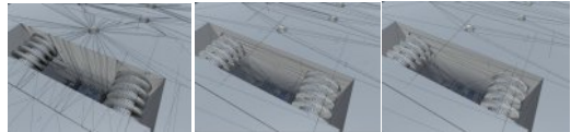
(a) High(30k Tri) (b) Middle(11k Tri) (c) Low(8k Tri) Fig. 7 Compare meshes based on tessellation level
