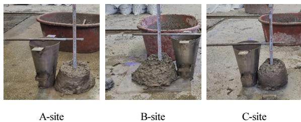
Fig. 2. Photos for concrete slump test
