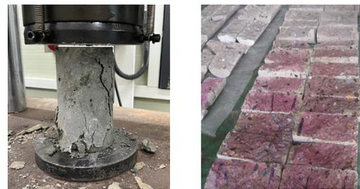
(a) Compressive strength (b) Carbonation test
