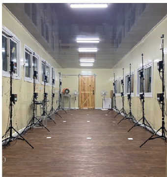
Figure 1 (a) Schematic diagram and (b) production of indoor simulation chamber for particulate matter suspension experiment
