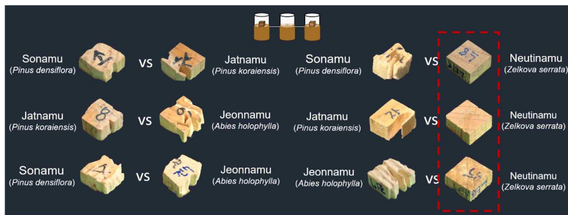
Fig. 3. Wood damage caused by Reticulitermes speratus in the two-choice test.
