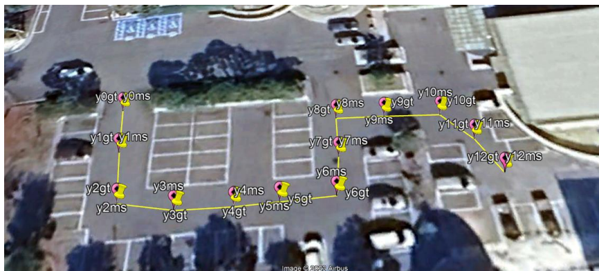
FIGURE 13. Trajectory Planning of an Autonomous Mobile Robot for HPE Testing
