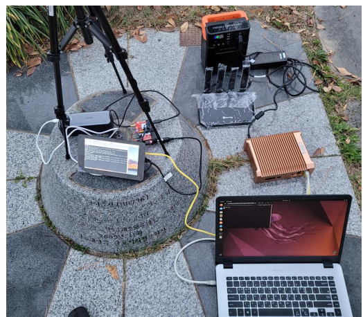
FIGURE 7. Test environment for fixed position points of precision positioning processing module
