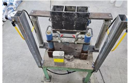
Fig. 3. Vibration Molding (1800 RPM)
