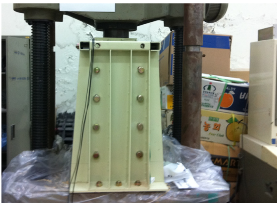
Fig. 7. The simulation test for the buried pipes
