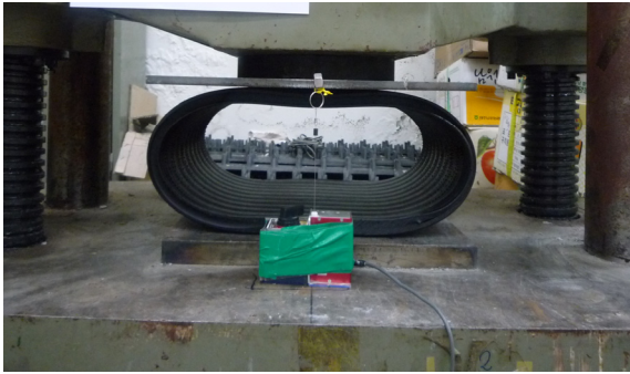
Fig. 3. Deformed shape of the PE pipe
