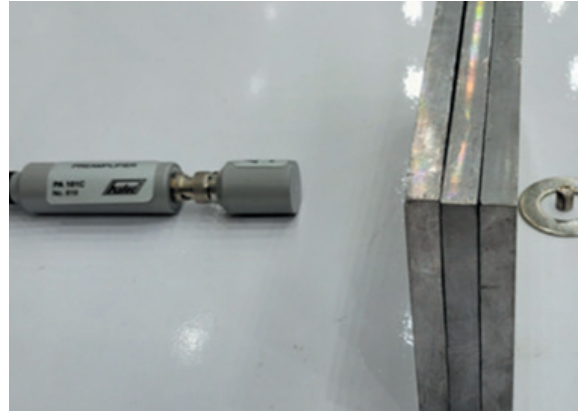
Fig. 2. Gamma-ray measurement experiment with lead shielding.
