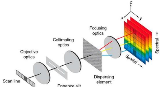
Fig. 8 Optical chain of a common imaging spectrometer (Srivastava et al., 2009)
