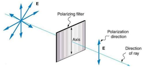
Fig. 7 A polarizing filter(voer.edu.vn)
