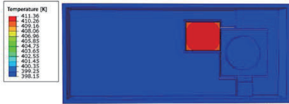
Fig. 7 Steady-state thermal analysis for TR module with high temperature case (398 K)
