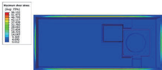
Fig. 12 Maximum shear stress contour
