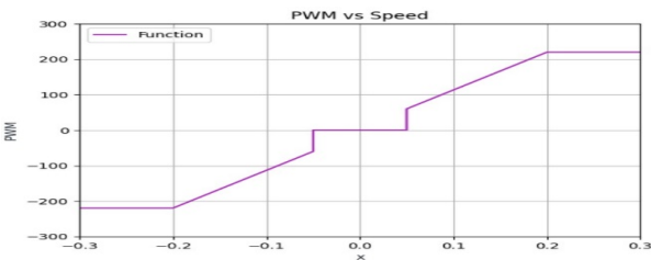
[Fig. 5] PWM signal correlation with speed
