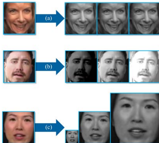
Fig. 1. Differences in grayscale images by key components: (a) RGB-to-grayscale conversion, (b) brightness level, and (c) resolution level
