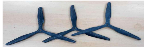
Fig. 13. Propellers made of composite materials
