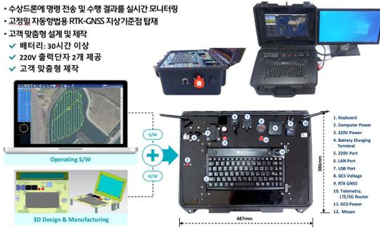
Fig. 8. Ground control system and operating S/W on GCS.
