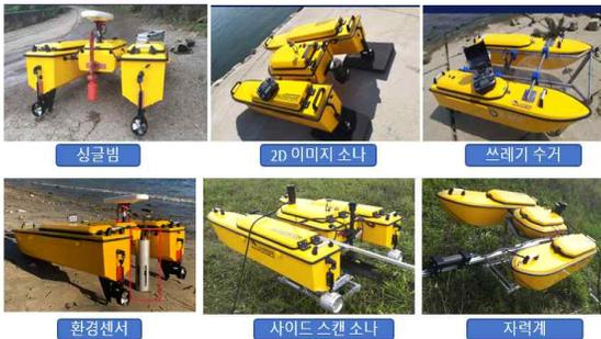
Fig. 2. USV with catamaran structure for various purposes (Model : GEOSONAR-300)
