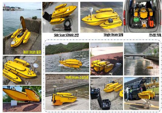
Fig. 3. USV with catamaran structure for Multibeam echo sound (Model : GEOSONAR-400)
