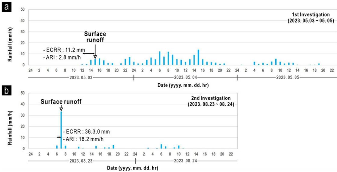
Fig. 4. Temporal rainfall distribution and occurrence timing of surface runoff during rainfall events in Josu-ri Sumgol area. The (a) 1<sup>st</sup> and (b) 2<sup>nd</sup> rainfall events (ECRR: Effective Cumulative Rainfall for Runoff, ARI: Average Rainfall Intensity).
