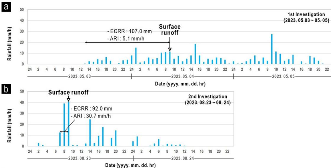
Fig. 5. Temporal rainfall distribution and occurrence timing of surface runoff during rainfall events in Geumak-ri Sumgol area. The (a) 1<sup>st</sup> and (b) 2<sup>nd</sup> rainfall events (ECRR: Effective Cumulative Rainfall for Runoff, ARI: Average Rainfall Intensity).
