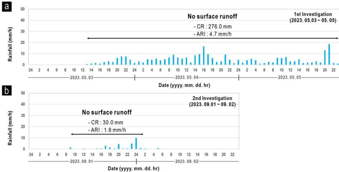
Fig. 6. Temporal rainfall distribution and occurrence timing of surface runoff during rainfall events in Songdang-ri Sumgol area. The (a) 1<sup>st</sup> and (b) 2<sup>nd</sup> rainfall events (CR: Cumulative Rainfall, ARI: Average Rainfall Intensity).
