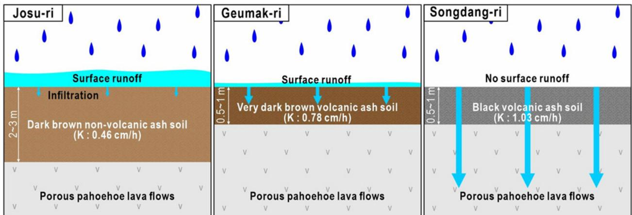
Fig. 8. Schematic images of surface runoff occurrence in the Sumgol watersheds having different hydrogeologic conditions. (K: Hydraulic conductivity; Park and Kang, 2019)
