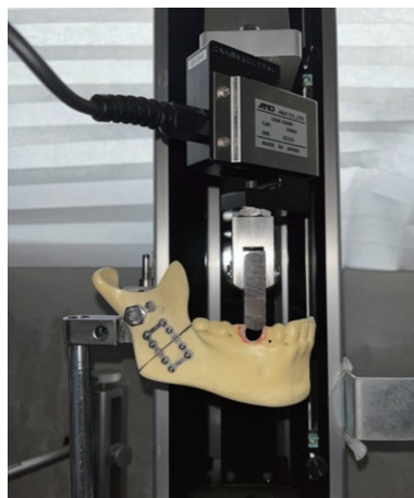
Fig. 2. Position of the polyurethane mandible on the force tester.
