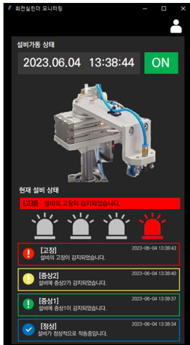
<Figure 7> Developed GUI Interface for Applying the Proposed Fault Detection Model in Remote Management Situation
