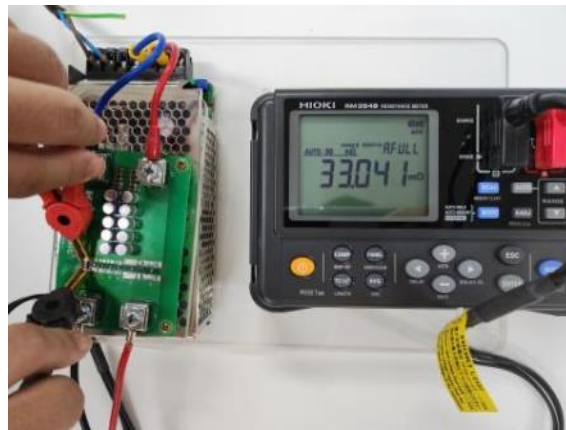
Figure 2. Internal resistance measurement using Hioki equipment
