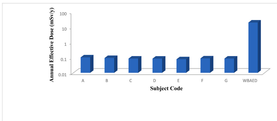
Figure-3. Comparison of Average Annual Effective Dose ( in vivo and in vitro Measurements) of workers with whole body Annual Effective Dose (in logarithmic scale).
