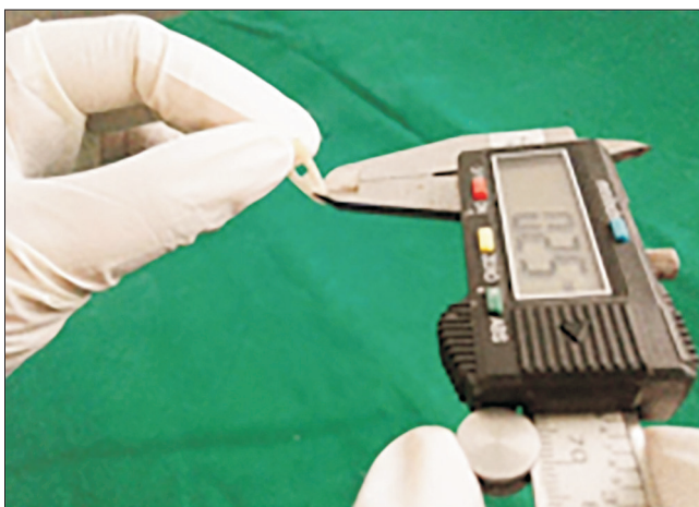
Fig. 1. Measuring the thickness of the section using digital vernier caliper.
