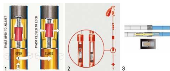
Fig. 3. Internal Structure of Climbing Stick[10]
