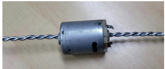
Fig. 8. power generator inside a climbing stick
