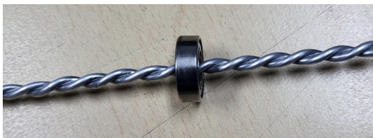
Fig. 7. device that converts linear motion into rotational motion
