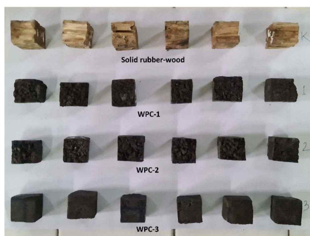
Fig. 4. Test specimens exposed to subterranean termites. WPC: wood plastic composite.
