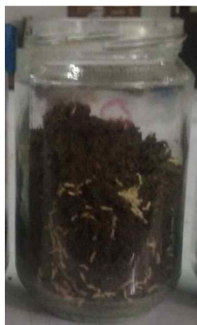
Fig. 2. A no-choice WPC termite test against subterranean termites in the laboratory. WPC: wood plastic composite.
