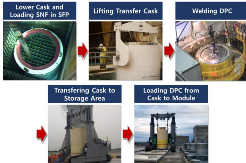
Fig. 4. Operation procedure of vertical storage module-based dry storage method
