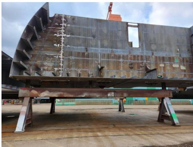
Fig. 1. A example of block supported by A-typed carrier.
