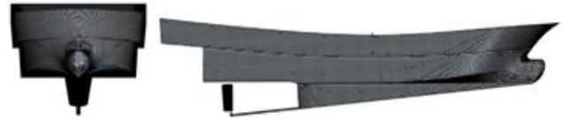
Fig. 5. Fishing vessel (4.99ton) Mesh Grid.
