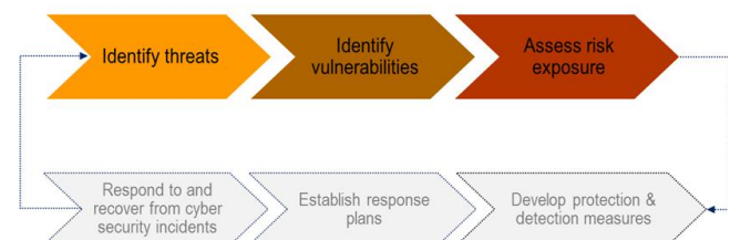
Fig. 1. Cyber risk management approach as set out in the guidelines by BIMCO and others (BIMCO et al., 2020).
