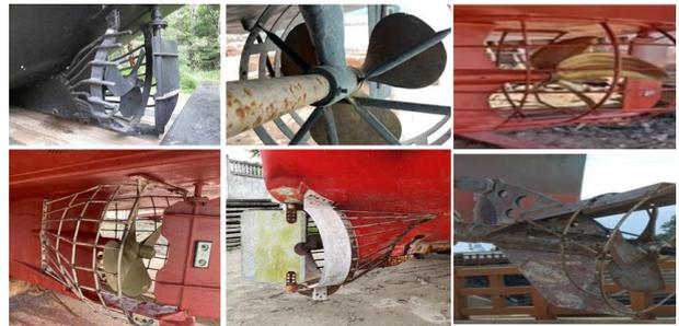
Fig. 2. Types of Inboard Motor Propeller Guards.
