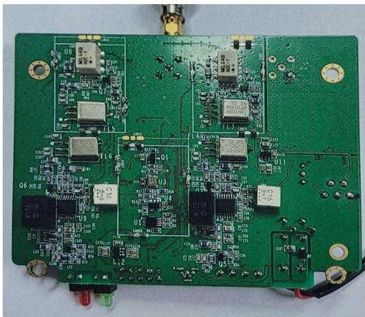
Fig. 13. Class B AMRD Receiver.
