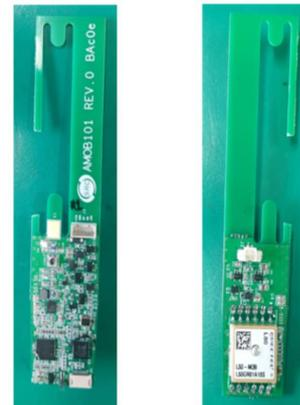
Fig. 8. Front and rear PCB / manufactured MOB-AIS Tx.
