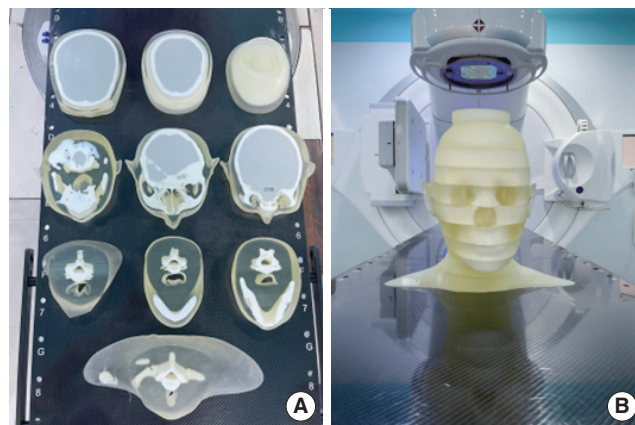
Fig. 3. A human body phantom fabricated using a three-dimensional printer. (A) Head and neck phantom divided into 10 layers. (B) Head and neck phantom with single-layer assembly.
