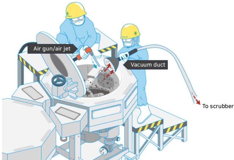
Figure 2. Recommended integration of air-gun and vacuum duct for effective dust removal
