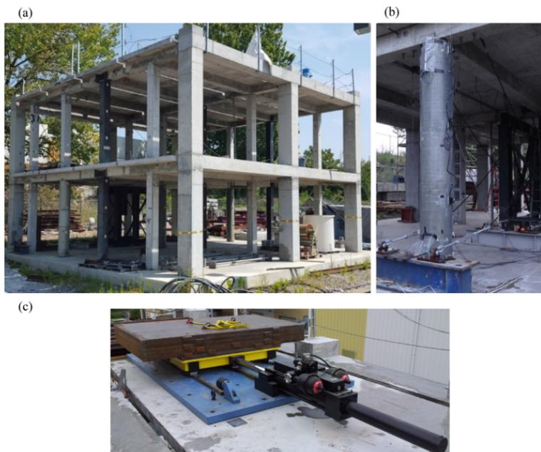
Fig. 2. Full-scale, two-story two-bay non-ductile RC test frames: (a) Four identical full-scale test frames; (b) FRP jacketed column in retrofitted test frame; (c) Hydraulic linear shaker used in the dynamic testing program
